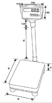
**Dimensions and Capacity (All measurements are in mm):**
